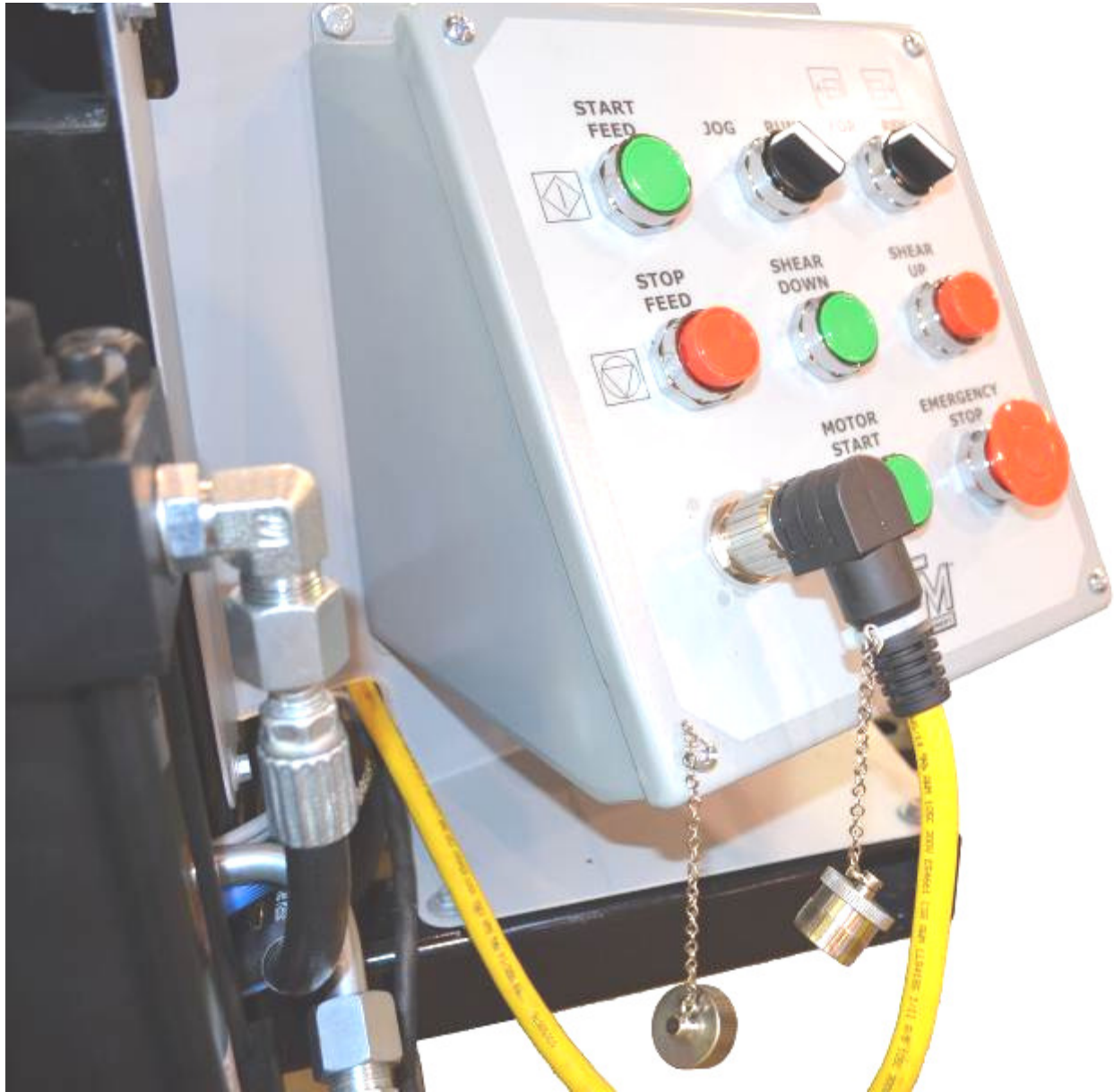
Figure 6: Main Control Cable
