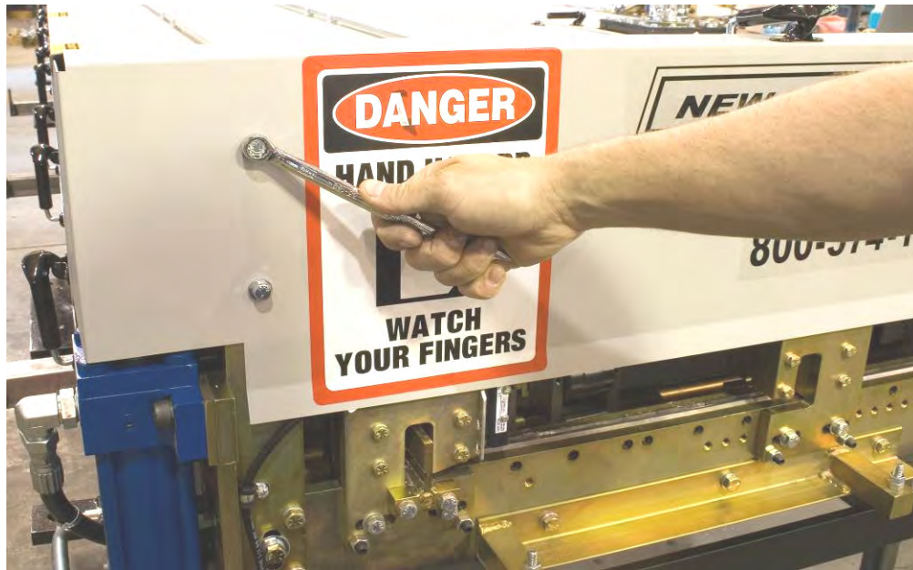
Figure 56: Removing Shear Cover
