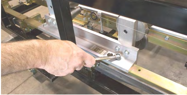
Figure 38: Removing Tooling Rails
