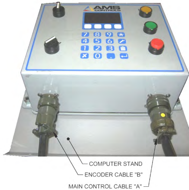
Figure 87: AMS Box With Cables
