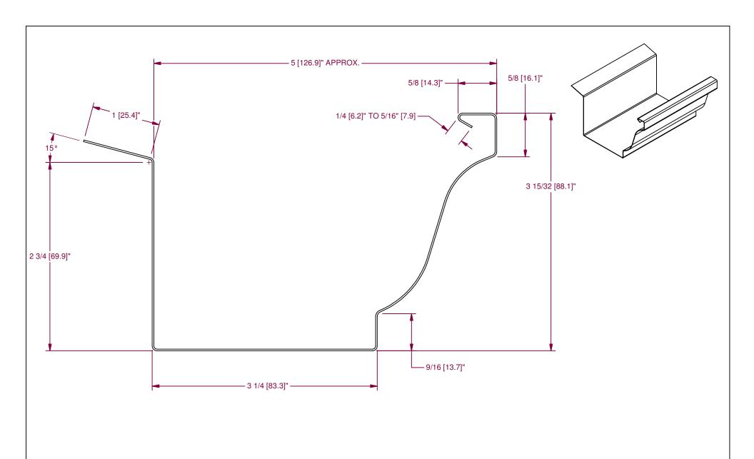
NOTE: 1. COIL WIDTH: 11 3/4" [298mm] to 11 7/8" [302mm] 2. DUAL DIMENSIONS: Inch [mm]
